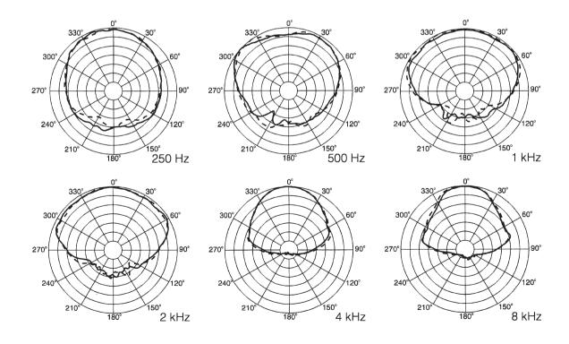
*Figure 1, One-Third-Octave Polar Response Charts Measurements were made in a 1.5 ft<sup>3</sup> closed enclosure.*
